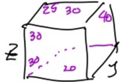
$$F(x, y, z) = \underbrace{25xy}_{\text{top}} + \underbrace{20xy}_{\text{bottom}} + \underbrace{30(xz + xz + zy)}_{\text{sides}} + 40zy$$
